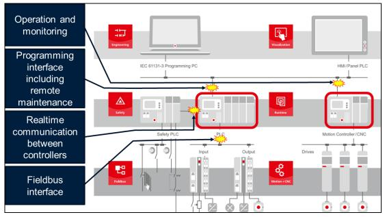
Figure 1: Possible vulnerabilities in a typical automation environment
